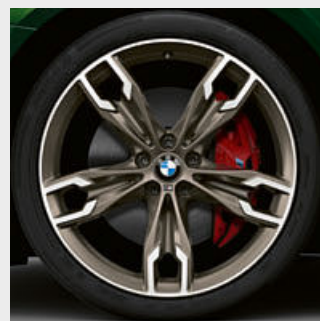
□ 20" M light alloy wheels Double-spoke style 668 M Cerium Grey matt with mixed tyres and runflat tyres, gloss-lathed, wheel size front 8J x 20 with 245/35 R20 tyres, wheel size rear 9J x 20 with 275/30 R20 tyres. 3
