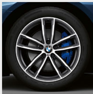
□ 18" M light alloy wheels Double-spoke style 662 M Bicolour Orbit Grey, gloss-lathed, wheel size 8J x 18 with 245/45 R18 tyres. 2
