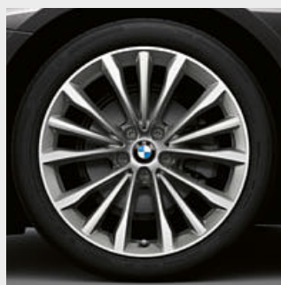
□ 19" light alloy wheels W-spoke style 663 Ferric Grey gloss-lathed with mixed tyres and run-flat properties, front 8J x 19 with 245/40 R19 tyres, rear 9J x 19 with 275/35 R19 tyres.
